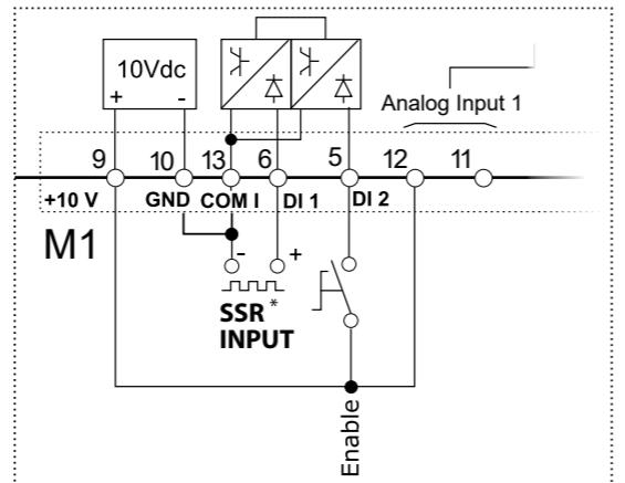
\* SSR Input: 4 ÷ 30Vdc 5mA Max (ON >4Vdc OFF <1Vdc)
