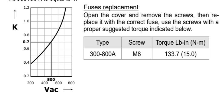
⚠ Caution: High speed fuses are used only for the thyristor protection and can not be used to protect the installation.
