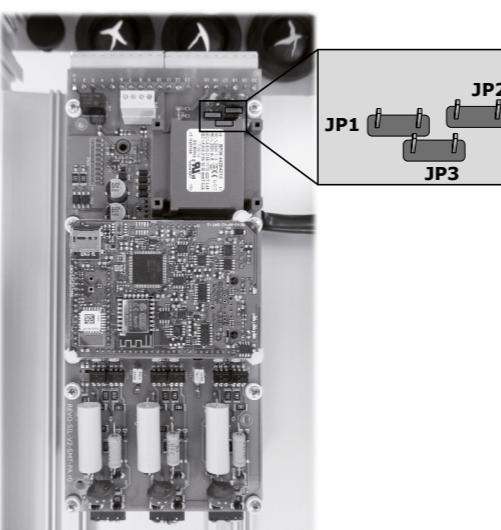
To change auxiliary supply voltage sold the correct link-jumper on REVO S board, the type of mounted transformer depends of the chosen Voltage in the order code.
