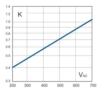
\* I2T are multiplied for K value in function of Vac at 500V K is equal to 0,7 (750 X 0,7 = 525 1800 X 0,7 =1260).
