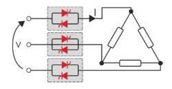
Delta wiring with resistive load (control on three phases)
