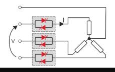
Delta wiring with resistive load (control on three phases)
