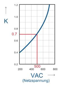
\*I2T are multiplied for K value in function of Vac at 500V K is equal to 0,7 (ex:15400 X 0,7 = 10780). At 660Vac K is equal to 1.
