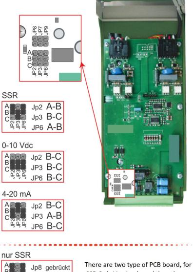
There are two type of PCB board, for SSR Only Version board the other jumpers are not mounted on PCB.
